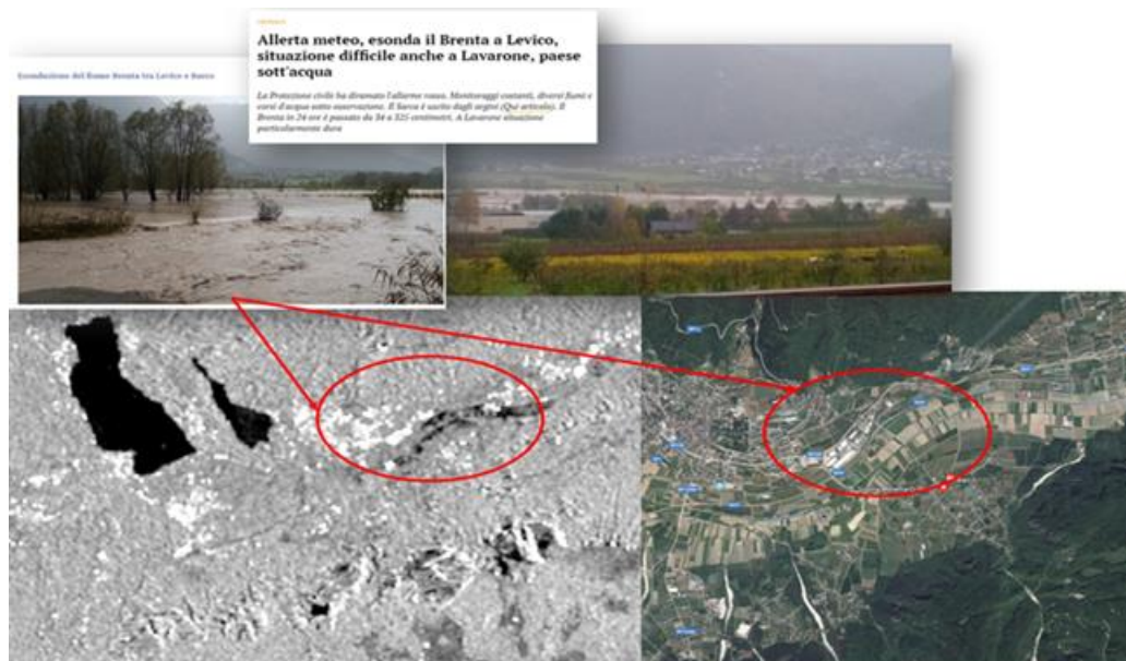
Figure 14: Flood detection products generated by AAWA pre-platform (November 2018)
