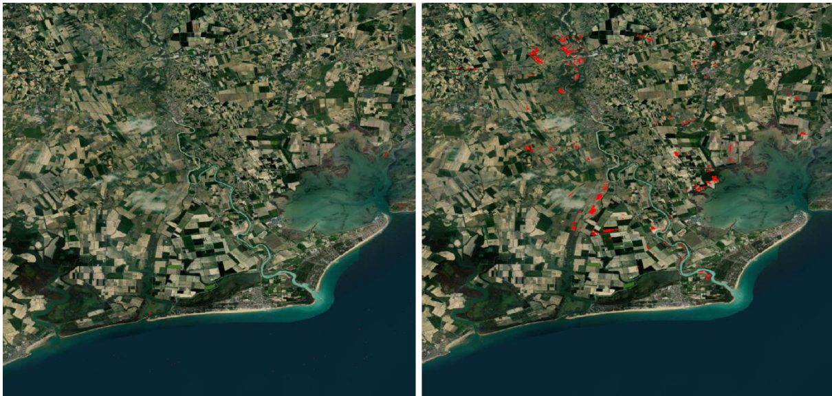
Figure 5: Flood map of Lemene river region on 15/11/2019, at a dry state (left) and on 17/11/2019, during a flood event (right). Flooded areas appear in red colour.
